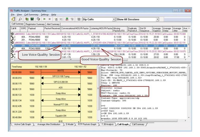
Measuring delay, jitter, packet loss, and voice quality through ATM/IP networks is very important. GL offers powerful features within **PacketScan™** software to capture and monitor live signaling and traffi-c. PacketScan<sup>™</sup> can capture, decode, segregate, monitor, and collect statistics on all Ground-to-Ground calls and Air-to-Ground calls as per EUROCAE ED-138 standards. The PacketScan<sup>™</sup> is an essential tool for troubleshooting and passive monitoring.
