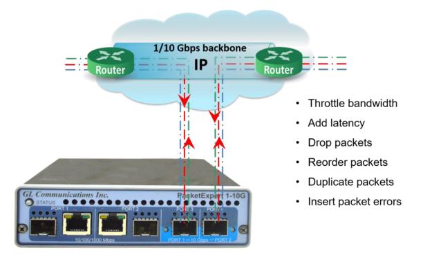
GL can simulate real world WAN impairments in order to safely test applications in the lab.
